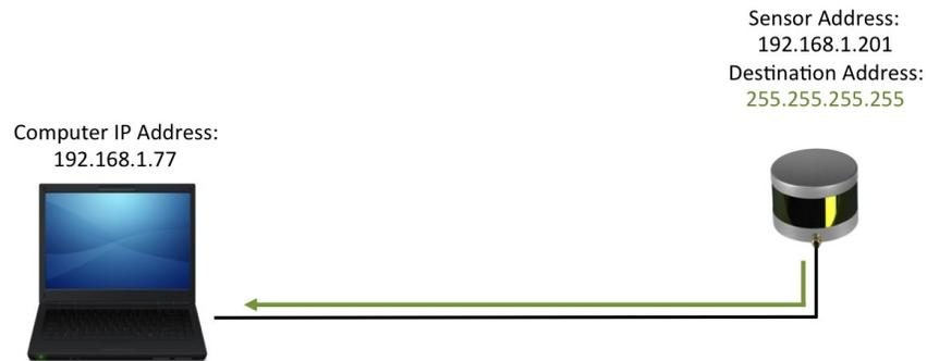
This is the simplest network, with sensor data flow free from competition or interference. Here it is acceptable for the sensor to broadcast its data on the network.
