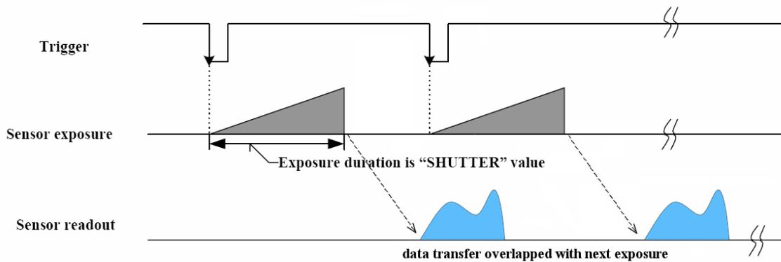
Figure 7.3: Trigger Mode 14 (“Overlapped Exposure/Readout Mode”)
