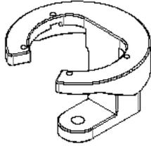
The tripod adapter attaches to the bottom of the camera.
