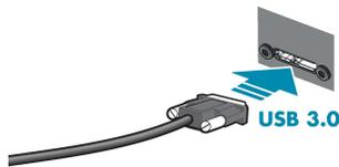
Plug the USB3 cable into the camera and secure with the cable jack screws. Using jack screws ensures a reliable connection and the pressure of the seal helps to keep moisture out of the camera.
