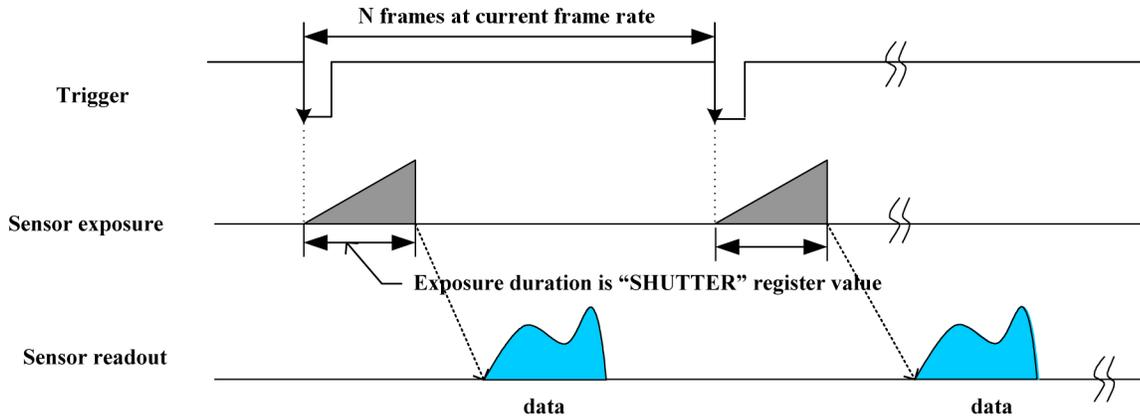
Figure 7.2: Trigger Mode 3 (“Skip Frames Mode”)
