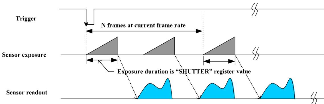
Figure 7.4: Trigger Mode 15, when  $N$  is greater than 0. (“Multi-Shot Trigger Mode”)
